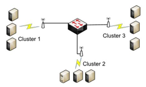
Figure 2: Network Architecture Structure for Fly-by-Wireless Systems
